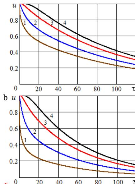
Fig. 5. Change in time of dimensionless moisture content sabrefish: 1) on the sample surface ( $x = 1$ ); 2)  $x = 0.8$ ; 3)  $x = 0.5$ ; 4)  $x = 0.0$ ; a)  $T=20^\circ\text{C}$ ,  $d = 10.8$  g moisture per kg dry air; b)  $T=30^\circ\text{C}$ ,  $d = 7.4$  g moisture per kg dry air
