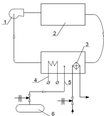
Fig. 1. The scheme of experimental installation: 1 – fan; 2 – drying chamber; 3 – cooler; 4 – electric heater; 5 – humidifier; 6 – steam generator
