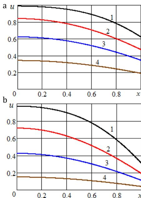
Fig. 4. Profiles of the dimensionless moisture content sabrefish at different points in time: 1)  $\tau = 10$ ; 2)  $\tau = 30$ ; 3)  $\tau = 60$ ; 4)  $\tau = 120$ ; a)  $T=20^\circ\text{C}$ ,  $d = 10.8$  g moisture per kg dry air; b)  $T=30^\circ\text{C}$ ,  $d = 7.4$  g moisture per kg dry air
