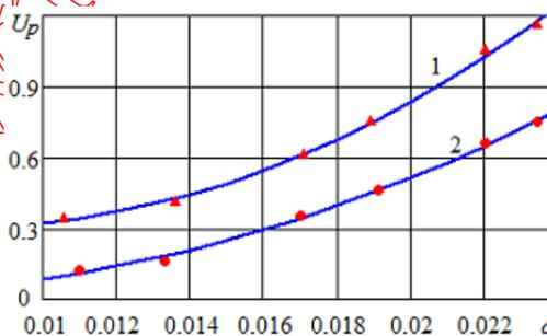
Fig. 3. Dependence of the equilibrium moisture content of herring (kg of moisture per kg of dry matter) from the moisture content of the air (g moisture per g of dry air) at  $T = 30^\circ\text{C}$ : 1 – whole fish, 2 – pieces. Points – experimental data; curves: calculation formulas (10)-(11)
