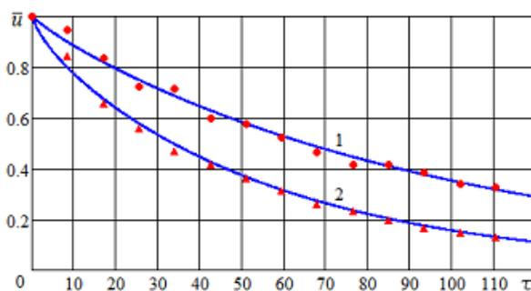
Fig. 6. Curves of dehydration during drying sabrefish in the period of falling speed (dimensionless variables): 1)  $T = 20^\circ\text{C}$ ,  $d = 10.8$  g moisture per kg dry air; 2)  $T = 30^\circ\text{C}$ ,  $d = 7.4$  g moisture per kg dry air. Points - experimental data, lines - result of calculation
